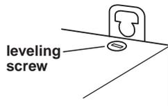
**13.** Use a flat-blade screwdriver and tighten the two leveling screws located close to the mounting brackets.
